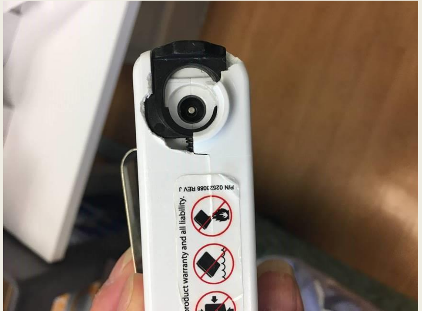
Battery locking mechanism broken
